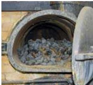
Inside the airtight retort coal was \_\_\_\_\_ at temperatures of 1200°C. The process produced gas and turned the coal into \_\_\_\_\_. This was recycled as fuel to heat the retorts or sold to local houses and factories.
